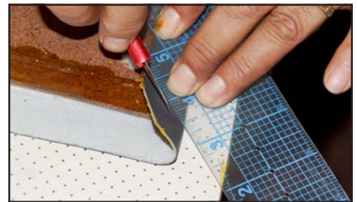
Figure 8: Stay an 1/8 in from the edge when cutting diagonal relief cuts
