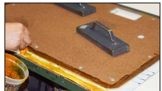
Figure 6: Apply contact cement to vinyl
