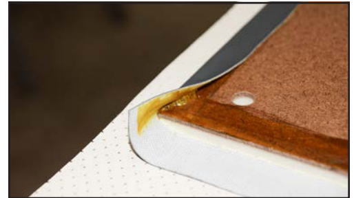
Figure 7B: Working the center to the corners, stopping before the edge
