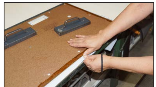
Figure 10: Gently pull the vinyl away from the top along the bottom edge
