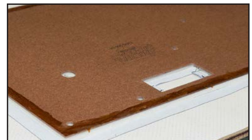
Figure 5: Apply contact cement to hardboard
