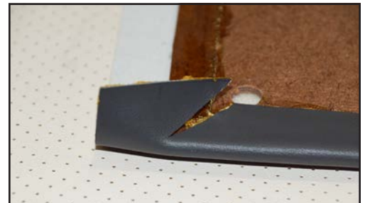
Figure 9: To achieve clean miters, leave excess until all 4 sides are attached
